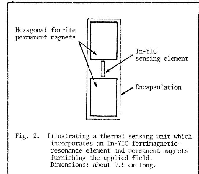
Fig. 2. Illustrating a thermal sensing unit which incorporates an In-YIG ferrimagnetic-resonance element and permanent magnets furnishing the applied field. Dimensions: about 0.5 cm long.
