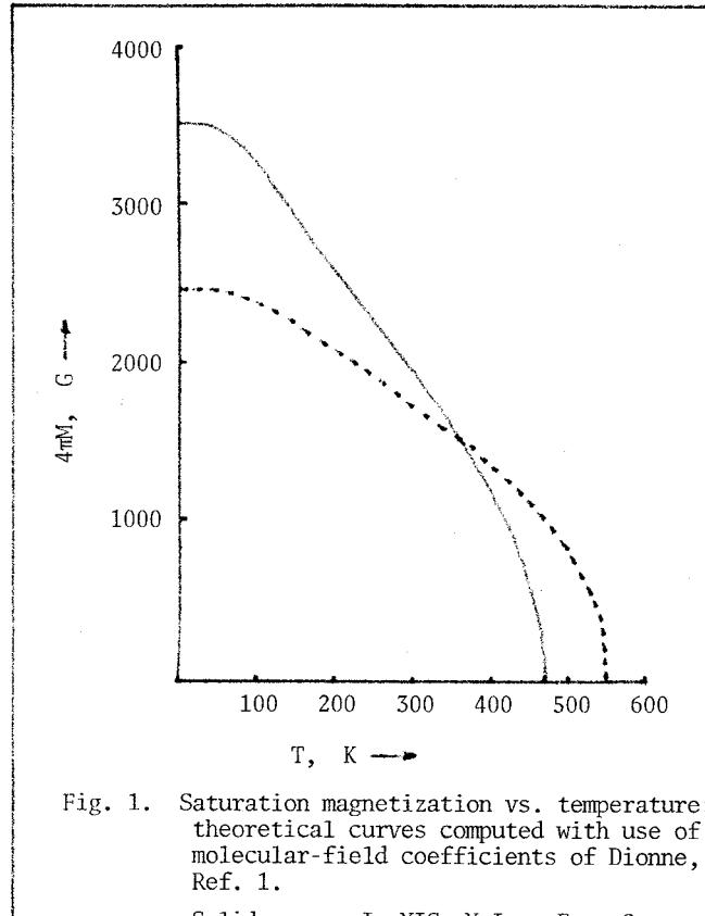
Fig. 1. Saturation magnetization vs. temperature; theoretical curves computed with use of molecular-field coefficients of Dionne, Ref. 1.
